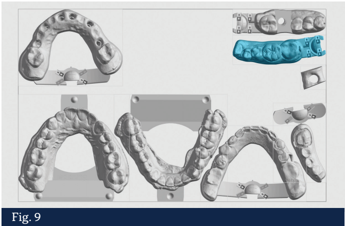
Building plate for digital model printing
